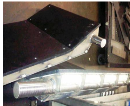
Diverter Flap TEFLON IMPACT Angle plus HD ROD with Foam Insulation
