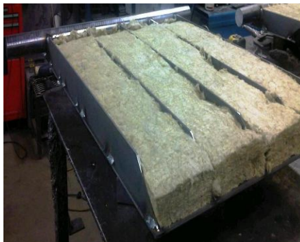
Diverter Flap RIBS plus Roxul Sound Dampening
